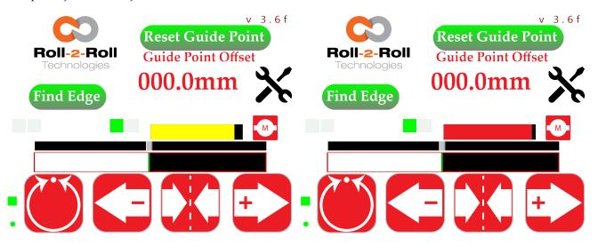
Figure 5.16: Actuator Extended Position Alert
