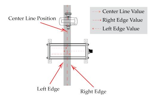
Figure 5.92: Centerline position of the web when using a single sensor that can detect both the left and the right edge.
