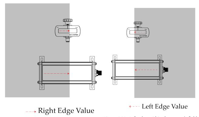
Figure 5.90: Left edge within the sensor's field of Figure 5.89: Right edge within the sensor's field view: output value increases as the web moves of view: output value increases as the web moves from right to left from left to right
