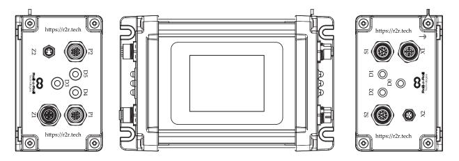
Figure 4.2: SCU6x controller Connector and Port Labels
