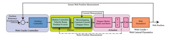
Figure 3.2: Control structure for Roll-2-Roll® Controllers for web guiding applications
