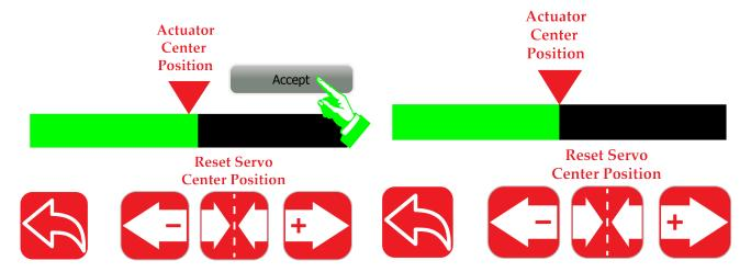
Figure 5.45: Accept the New Servo Center Position Figure 5.46: Save the New Servo Center Position as an Offset
