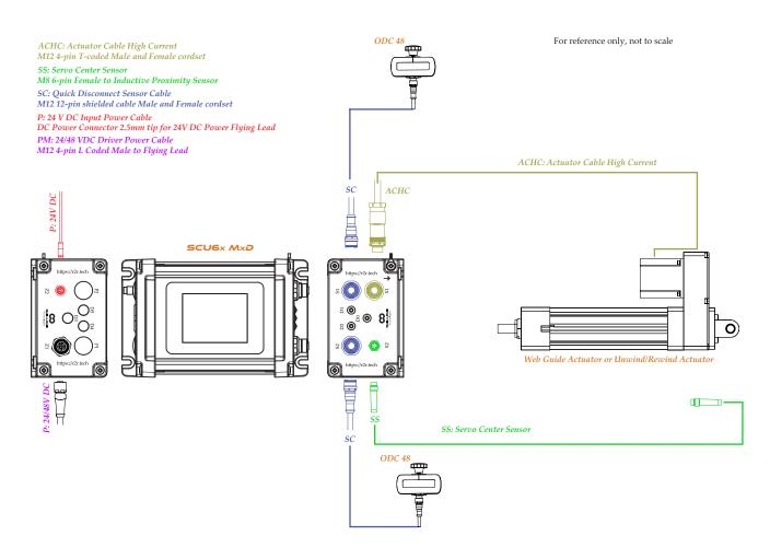
Figure 6.3: Wiring example with a unwind/rewind actuator.
