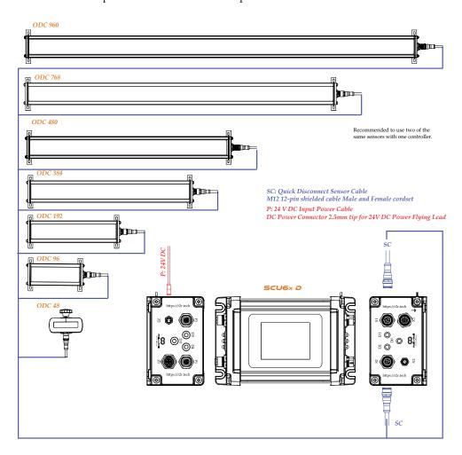
Figure 6.1: Wiring of the SCU6x controller for sensing and measurement applications.
