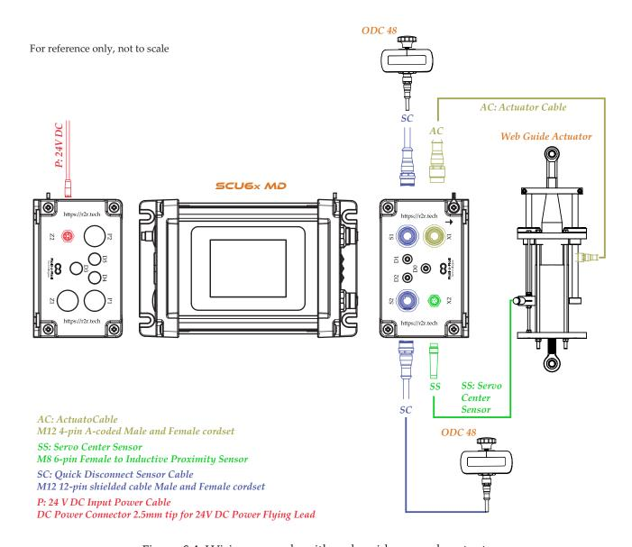
Figure 6.4: Wiring example with web guide upgrade actuator.
