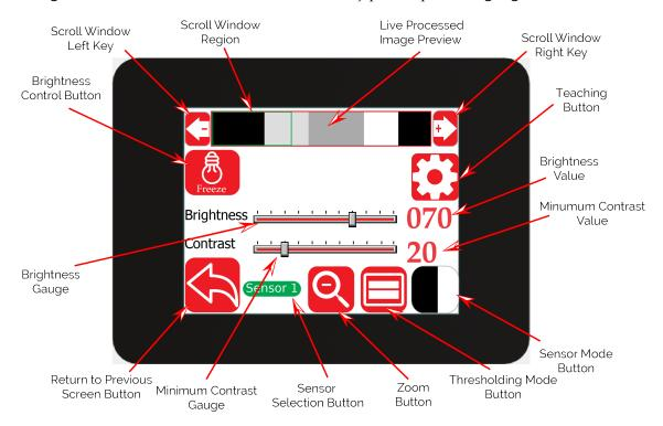
Figure 5.55: Operator Sensor Screen: Edge Mode
