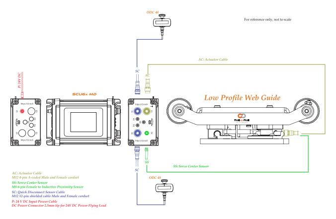
Figure 6.2: Wiring example with a displacement guide.
