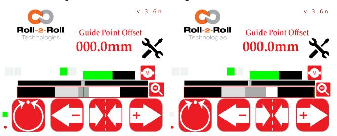
Figure 5.12: In the contrast mode, the real-time Figure 5.13: In the contrast mode, the real-time sensor image is shown on the web position bar. sensor image is shown on the web position bar.
