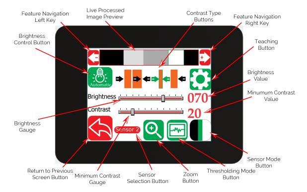
Figure 5.56: Operator Sensor Screen: Contrast Mode
