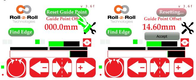
Figure 5.32: Guide point reset initiated by pressing Figure 5.33: Temporary guide point change based reset guide point button on the current web position is displayed
