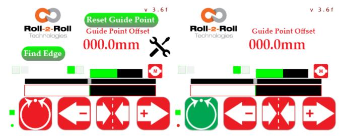
Figure 5.22: Controller in manual mode
