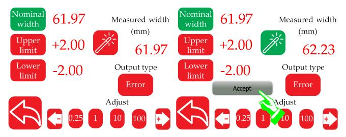
Figure 5.68: Teaching accepted by pressing the ac-Figure 5.69: Once teaching is accepted the offset is cept button applied to the measured width value
