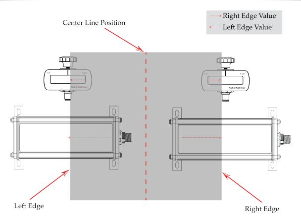
Figure 5.91: Centerline position of the web when using two sensors; one configured to left and the the other right.
