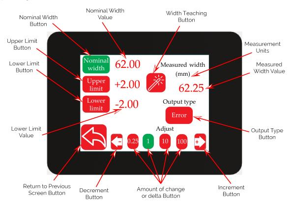
Figure 5.67: Operator Width Screen in mm
