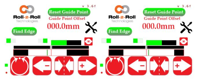
Figure 5.8: Sensor 1 left edge, Sensor 2 right edge. Figure 5.9: Sensor 2 left edge, Sensor 1 right edge.
