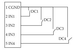
Figure 4.13: Typical wiring information for dry contact inputs
