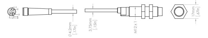
Figure 4.10: Servo center cable - Inductive Proximity Sensor (M12) with M8 Quick Disconnect
