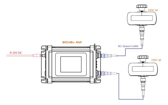
Figure 3.1: SCU6x Controller with two Roll-2-Roll® Sensors
