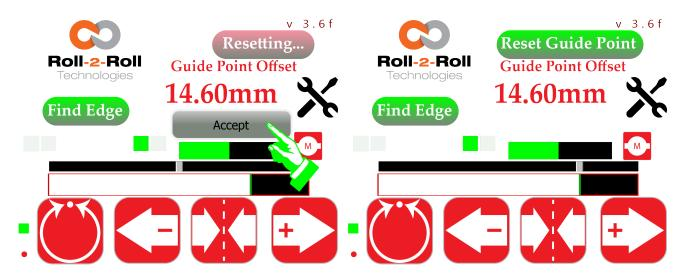
Figure 5.34: Temporary guide point not confirmed Figure 5.35: Gross guide change is confirmed and until the accept button is pressed accepted
