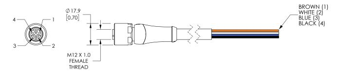
Figure 4.4: Driver Power Input Cable
