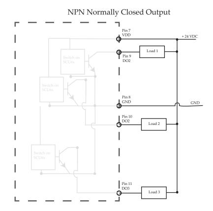
Figure 4.14: Typical wiring information for NPN normally closed output from SCU6x controller
