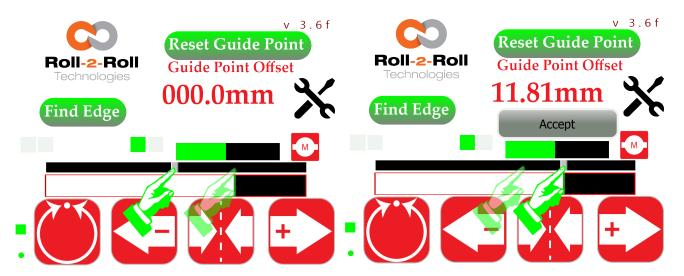
Figure 5.28: Gross guide point change by moving Figure 5.29: Release of track bar will prompt confirmation of the new guide point offset the track bar
