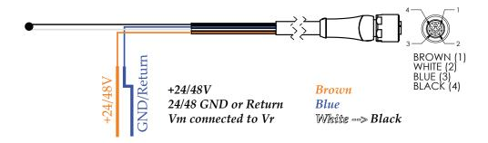
Figure 4.6: Driver Power Input Cable Wiring without Regen Clamp
