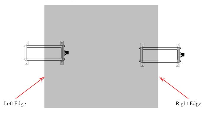
Figure 5.84: Proper sensor orientation for ODC 96 – ODC 960 and WPS 112 – WPS 900  $\,$
