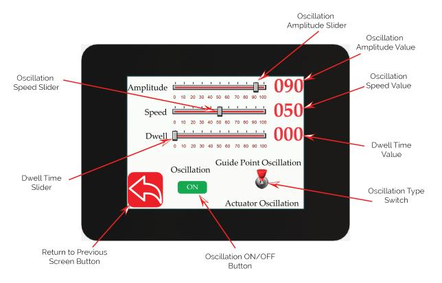
Figure 5.73: Operator Oscillation Screen
