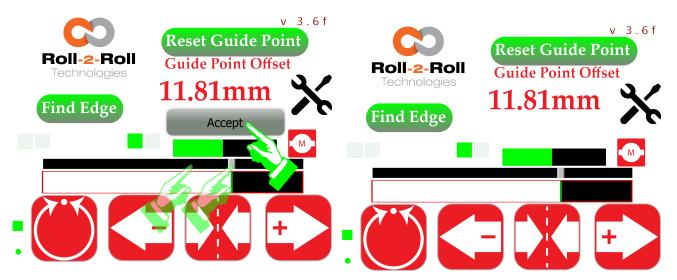
Figure 5.30: Gross guide point change needs to be Figure 5.31: New accepted guide point is confirmed accepted
