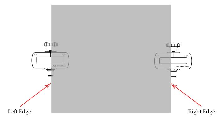
Figure 5.83: Proper sensor orientation for ODC 48 and WPS 48
