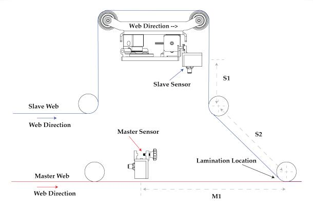
Figure 5.87: Master/Slave Sensor Installation Recommendation
