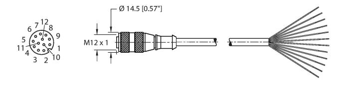
Figure 4.15: M12 12-pin Female to pigtail digital I/O cable
