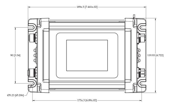
Figure 4.1: SCU6x controller Physical Dimensions (All dimensions are in mm [in]); Subject to change without notice.
