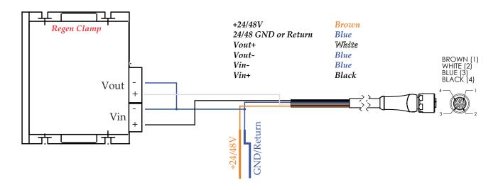
Figure 4.5: Driver Power Input Cable Wiring with Regen Clamp
